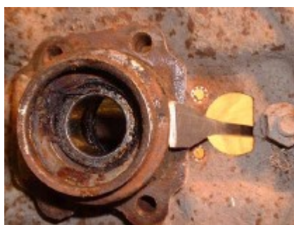
8. From the back side of the backing plate drive off the dust shield. Here I'm using a long handle gas-gasket scraper to catch the edge of the shield.
