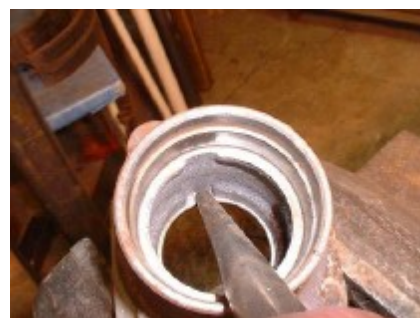
12. Use the slots in the hub to drive out the bearing cup. Walk it out by first hitting one side then the other until the cup walks out.
