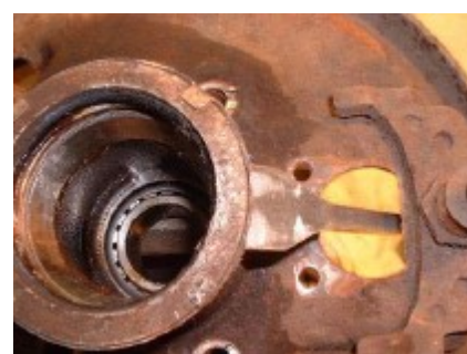
9. From the other side of the backing plate drive off the outer seal in the same manner as the dust shield in fig. 8.
