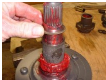
23. Slip the big spacer and the small shim over the axle shaft. If you didn't measure the shim thickness earlier now is your last chance.
