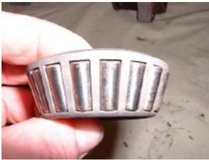
16. Although difficult to see in this photo this bearing has some very fine pitting. Always re-place all the bearings, cups and seals if possible.
