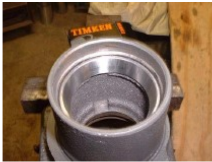
19. Drive the bearing cup all the way down until it contacts the bottom of the flange. Now flip the hub over and install the other bearing cup.
