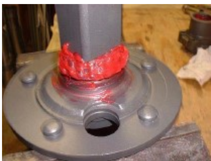
22. Be sure to put the bearing on the axle shaft in the right direction. Drive it down until it seats on the bottom.
