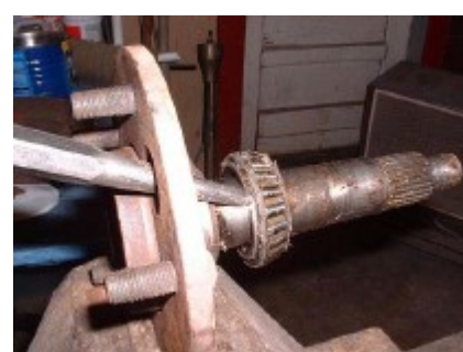
15. Once the bearing has moved enough use a long punch through the hole in the axle to drive it off the shaft.
