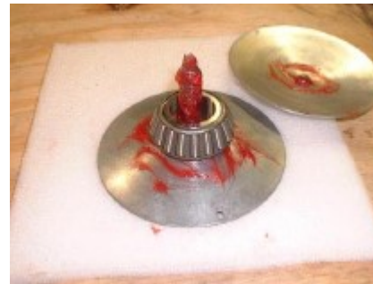
20. Here is one tool I recommend every DIYer own. A bearing packer uses a grease gun to force grease into the bearing much easier than by hand.
