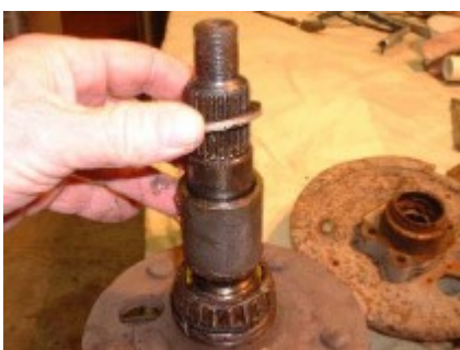
13. Measure the shim thickness with calipers or similar and record this reading. This is what sets the bearing preload and will be referenced later.
