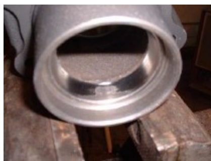
11. Here is an example of a bad bearing cup. Always replace both the cup and the roller together. This are too critical to leave to chance.
