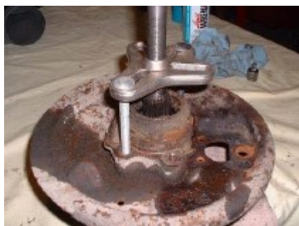
7. If the puller doesn't work this too will have to be pressed out. Keep the left and right side parts separate. Shims may not be the same thickness.
