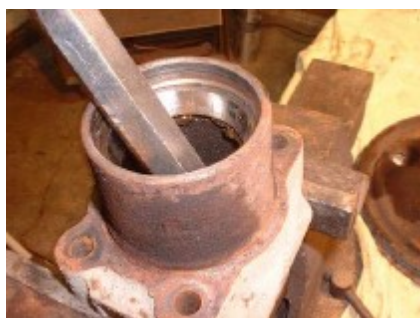
10. Drive out the inner bearing and seal with a large blunt chisel. Concentrate the blows on the center of the bearing and not the bearing cage.
