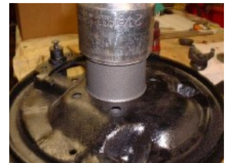
24. Slip the backing plate over the hub and install the outer seal. Use some type of driver, don't just drive it in with a hammer or you'll bend it.
